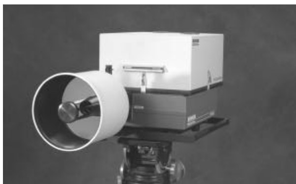
Figure 1 The MR254 spectrometer with the narrow-angle telescope mounted to it. In this picture it is standing on a tripod and is not mounted to the rest of the ScanSpec hardware. Published with permission from ABB Bomem.
