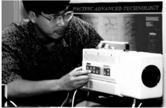
Figure 4 - The imaging spectrometer from Pacific Advanced Technology.
